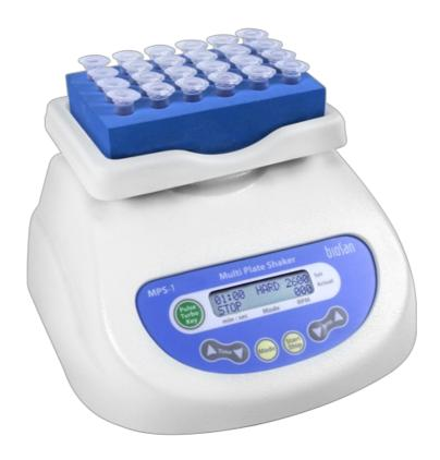
MPS-1 With built-in universal platform High—Speed Multi Plate Shaker
